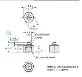
For details on sensor mounting bracket MS-DP1-1 and panel mounting bracket MS-DP1-2 / MS-DP1-4, please refer to "SUNX general catalog" or "DP-100 series catalog".
