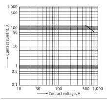
1-2.Max. switching capacity (DC resistive load)
