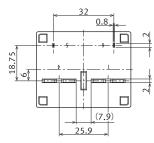
TOLERANCE; less than 10mm:  $\pm 0.3$  min.10mm~ :  $\pm 0.5$
