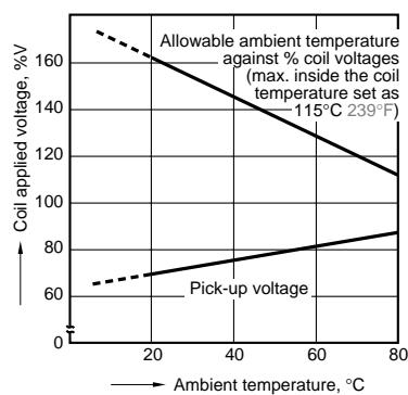
**4.- (2) Ambient temperature vs. coil applied voltage (High sensitivity type)**
