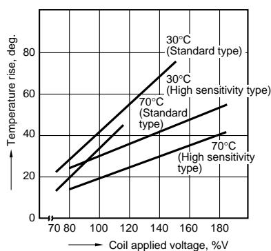
**4.- (1) Ambient temperature vs. coil applied voltage (Standard type)**
