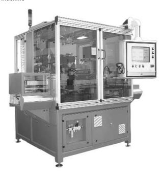
Automatic machine equipped with an insertion tool (comprised of productspecific insertion head, anvil, and product feed mechanism). Stepper-motor driven X-Y table positions PCBs under insertion head. Surface Mount Equipment Manufacturers Association (SMEMA) compatible inline PCB Insertion Station for posts, tabs, receptacles or sockets. Stand-alone unit is field upgradeable to Pass Through. Mounts up to four pneumatic insertion heads. Modem diagnostics standard, vision system optional.
