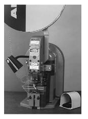
AMP-O-LECTRIC Model "K" Terminating Machine with a permanently-mounted applicator that accepts interchangeable die sets to apply a variety of tapemounted terminals and splices. Many of the die sets can also be used in AMP-O-LECTRIC Terminating Machines with a tape applicator.
