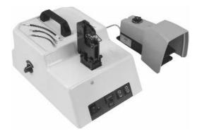
The SDE Electric Terminator applies a broad range of products, in the 6 - 0.3 mm<sup>2</sup> (10-22 AWG). This small, bench top power unit offers many features found on
