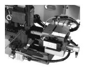
The combination of the Stripping Module with the AMP-O-LECTRIC Model G Terminator or the AMP 3-K/40, AMP 5-K/40 provides an economical, proficient method of stripping wire and crimping terminals on the same machine. Wires are stripped moments before crimping,
