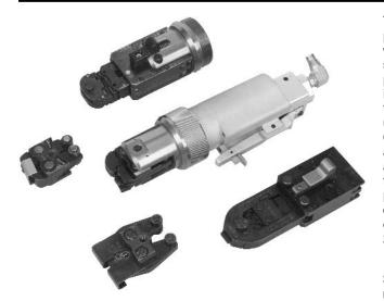
The new micro-pneumatic power unit provides minimal weight and minimal tool size, with maximum production. The power unit is compatible with the small tool and adapter holders used in the 6-26 system. Only available in a hand actuated version. This unit and compatible heads will terminate 26-14 AWG products, with the exception of the SOLISTRAND head combination, which crimps 22-10 AWG combinations.
