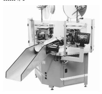
Fully-automatic machines that measure, cut, strip and terminate single leads. Microprocessor-controlled, and programmed and operated using an easy-tofollow, menu-driven touchscreen. Features include direct-drive terminating units with precision crimp height adjustment, fully programmable setups, wire runout and splice detection, and motorized pre-feed with wire straightener. Crimp quality monitoring is also available.
