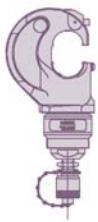
12 ton output force 1" stroke; 20,000 cycle Light Duty Compression Head 2 U-Die Compatible PN 1490745-1 IS 408-10111
