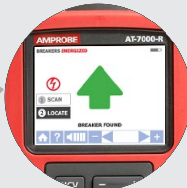
The solid green arrow and audible alert indicates the target breaker has been found.
