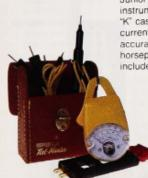
Junior Test Master Kits consist of a "YO" series instrument (measures amps, ohms and volts) in a "K" case with an A47-L Energizer to increase current measuring sensitivity by 10 times for accurate measurement of current on fractional horsepower motors and small appliances. Also includes clip-type leads with removable probe tips.
