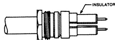
1. Place nut and gasket (w/v-groove facing forward) over cable jacket as shown. Trim braid and jacket to dimensions shown in Fig. 1. Comb out braid wires.
