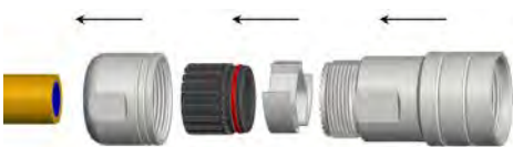
Step 1: Slide parts onto cable
