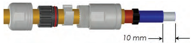
Step 6: Slide plug onto crimped terminal assembly
