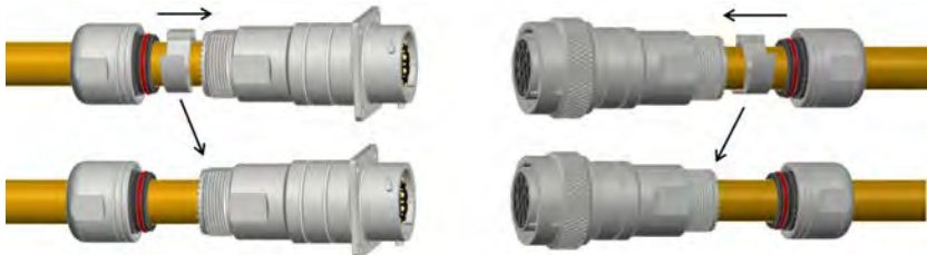
Step 11: Push shielding clip into backshell
