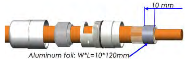
Step 4: Wrap foil over braided shielding
