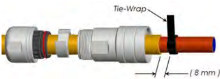
Step 3: Attach tie-wrap
