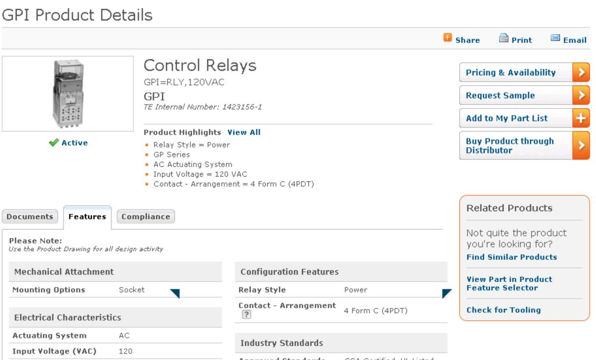
CSA Certified, UL Listed Approved Standards 10A Resistive @ 220 Contact Rating VAC/48 VDC RoHS/ELV Compliance Not ELV/RoHS compliant Lead Free Solder Termination Features Not relevant for lead free Processes 📳 process Termination Type 16 Flat Base Pins Conditions for Usage Dimensions Temperature Range 0 - 60**Approx. Dimensions (L**  $45.00 \times 45.00 \times 109.00$ (°C)  $\times W \times H$ ) (mm [in])  $[1.773 \times 1.773 \times 4.294]$ Other Series 🛽 GP Brand Agastat
