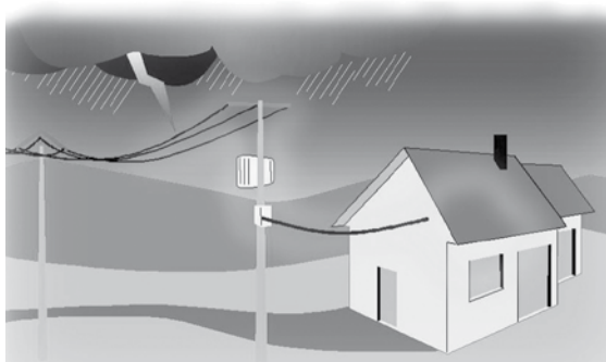
Direct lightning strike on an overhead line
