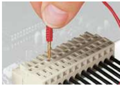
Testing perpendicular to conductor entry with 2 or 2.3 mm Ø test plug – female connector with CAGE CLAMP® – via integrated test ports
