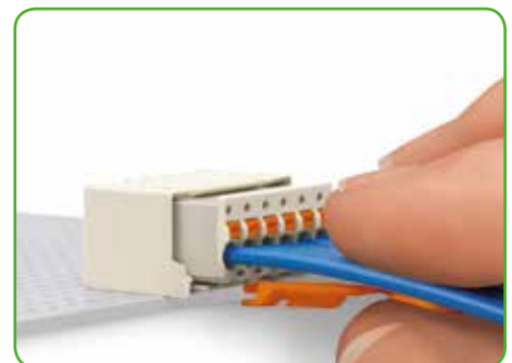
Pull on both unlocking tool and conductors to remove female connector from male header.
