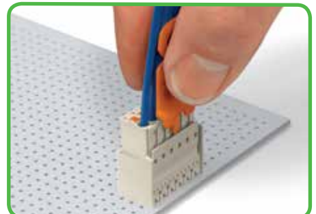
Pull on both unlocking tool and conductors to remove female connector from male header.
