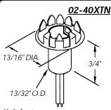
Unit features: Triple panel retention force. Elimination of an extra spacer. No loose parts.
