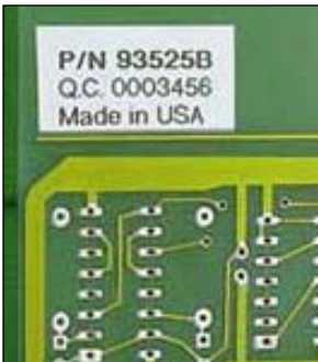
Circuit board labeling
