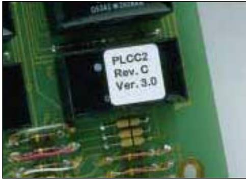
Circuit Board Labeling
