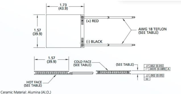
Ceramic Material: Alumina (Al<sub>2</sub>O<sub>3</sub>) Solder Construction: 271°C, Proprietary
