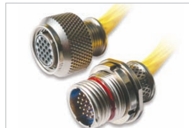
Connector uses size 23 contacts accepting #22 to #28 wire. Contact spacing is reduced to 0.076 inches providing a compact yet robust package.
