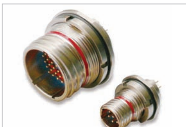
Double start threads prevent thread damage and allow full connector mating in 1.5 turns. Durable design ideal for harsh shock and vibration environments.
