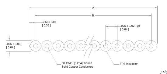
Note: Blue marking on one edge of cable designates wire #1.
